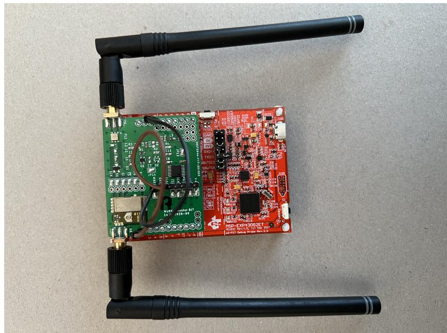
**Figure 3.** Wake-up Receiver equipped sensor node used in this work.
